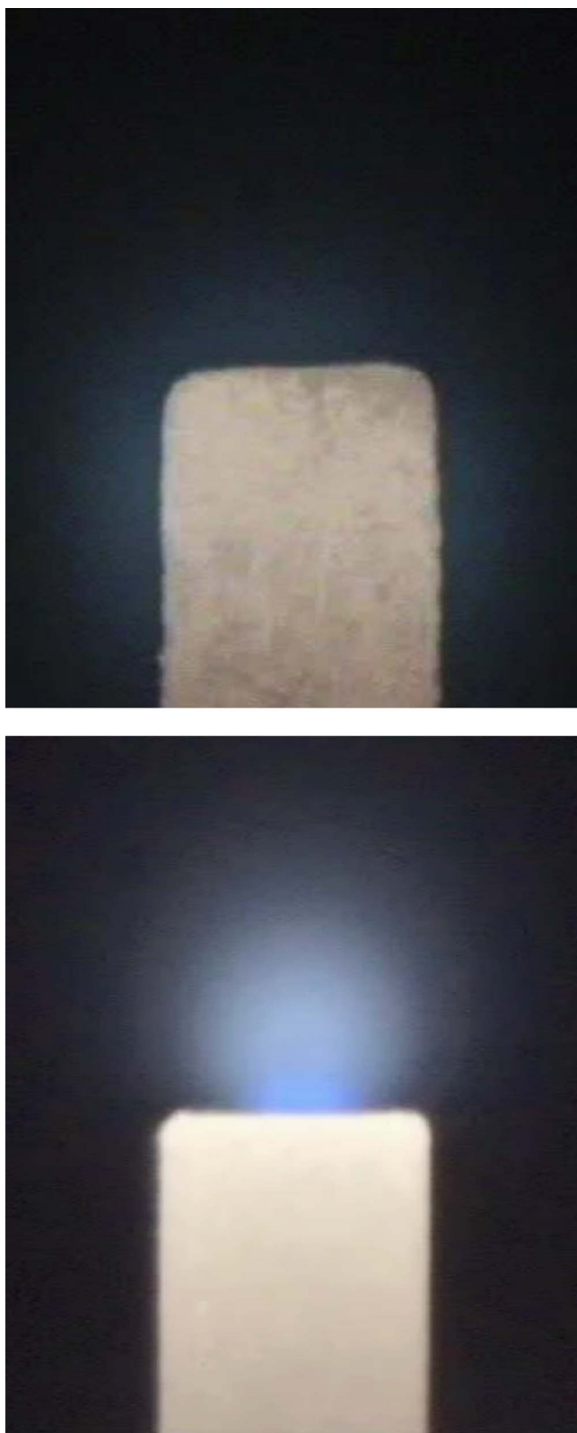
FIG. 1. (Color online) Pictures of the cathode region in the diffuse mode (left) and the hot-core mode (right). The cathode diameter was 0.6 mm and the arc current was 12.5 A in both cases.
